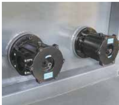
自封式过滤装置 Suction Filter With Check Valve
