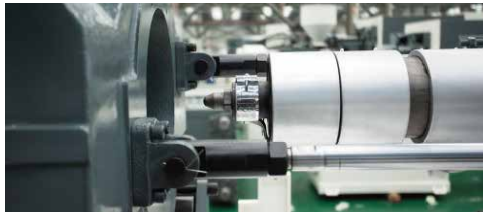
双射移油缸 Balanced Twin Cylinder Injection System
